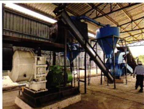
Torrefied biomass pellet manufacturing reactor, HPGCL-Hissar, Haryana
